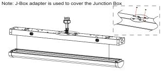
4. Turn off the power and make wiring by using wire nuts according to wiring diagram
