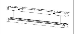
3.Run the fixture's power wires through the center hole. of the round J-box adapter. Slide and secure the round J-Box adapter on the center slots located on the back of the
